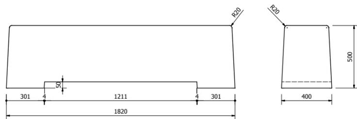
> Lg. 1820 x l. 400 x ht. 500 mm ⚖️ 750 Kg (estimation)
