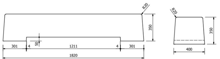
> Lg. 1820 x l. 400 x ht. 350 mm ⚖️ 500 Kg (estimation)
